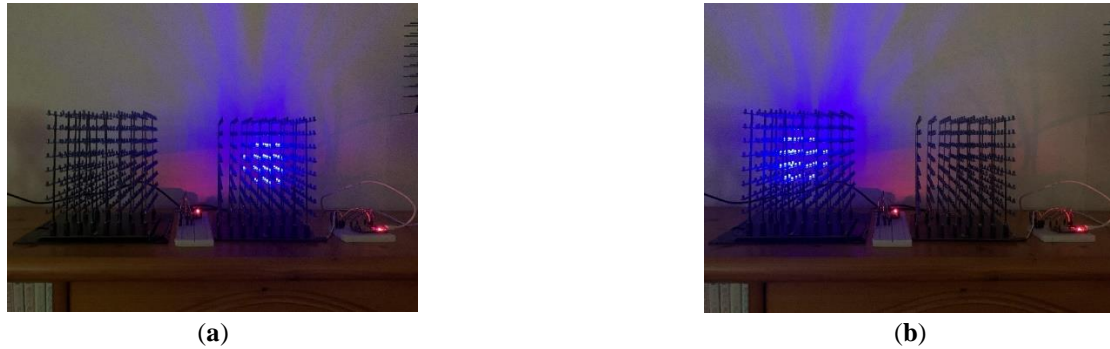
Fig. 10. LED cubes present interactive content where the blue lights moves from (a) the right side to (b) the left side, corresponding to the 3D ball track in RLDS.
